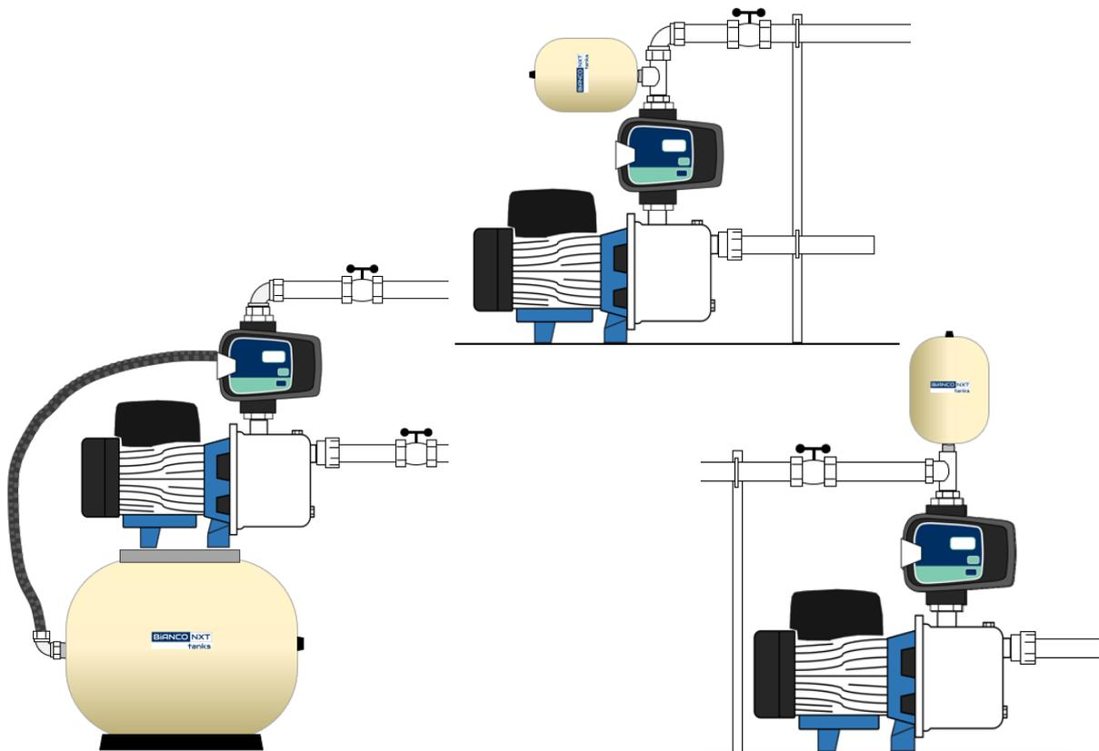
Note the Pressure controllers switch off at minimum flow which is close to maximum pump pressure.
